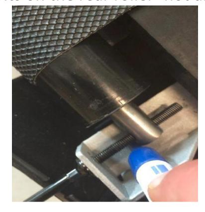
3. Remove the roller adjustment bolt(s).
