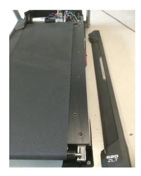
2. Tip: Use a permanent marker and mark the roller positions on the bolt on the front roller and bolts on the rear roller- not all front rollers
