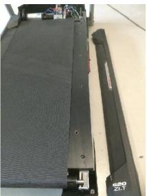
2. Tip: Use a permanent marker and mark the roller positions on the bolt on the front roller and bolts on the rear roller- not all front rollers have this adjustment bolt.
