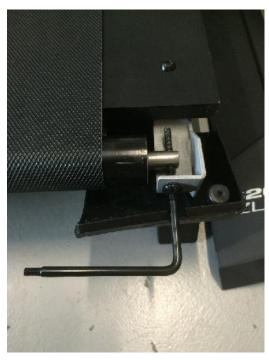
4. Remove the roller adjustment bolt(s).
