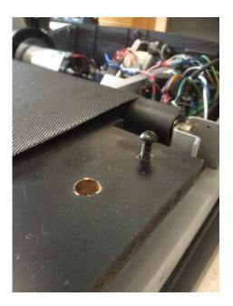
6. Remove the old walking belt, lift up the running deck and pull the belt out on the right side.
